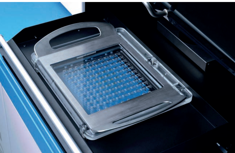
Fig. 3: The Trioptics OptiSpheric IOL PRO 2 in-situ production tray for 100 lenses.
