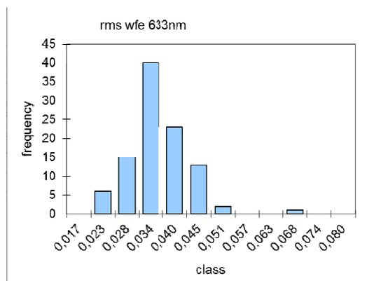
Figure 10 – RMS wavefront performance at 632.8 nm predicted by Monte Carlo analysis
